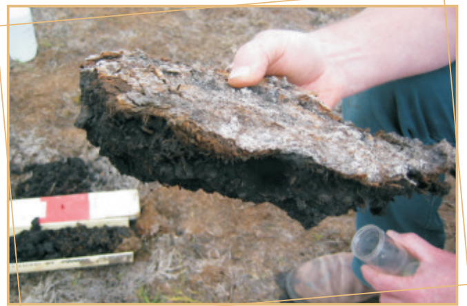
A CRC LEME student digs up an acid sulfate soil section for sampling.
